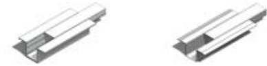
Omega + Tapeta Extrusionada Aluminium joint + cover plate Omega + Tapeta de acero Steel joint + cover plate
